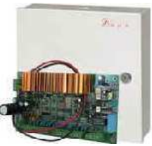
F-206/F-208/ F-216/F-448 Control Panel
